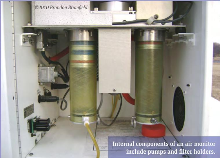
Internal components of an air monitor include pumps and filter holders.
